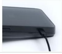
2. Insert the micro-USB connector into the USB port on the left side of the terminal.
